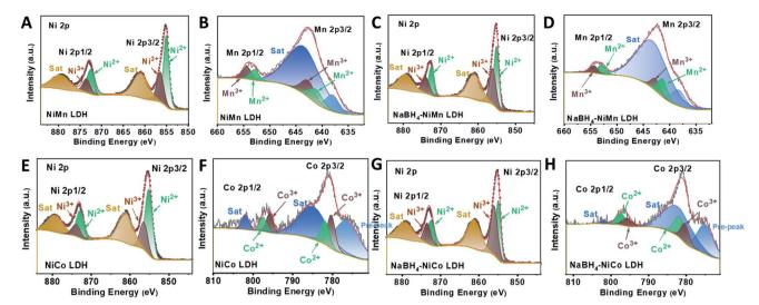
Fig. 4 High resolution XPS spectra of Ni2p for (A) NiMn LDH and (C) NaBH<sub>4</sub>-NiMn LDH; Mn2p for (B) NiMn LDH and (D) NaBH<sub>4</sub>-NiMn LDH; Ni2p for (E) NiCo LDH and (G) NaBH<sub>4</sub>-NiCo LDH; Co2p for (F) NiCo LDH and (H) NaBH<sub>4</sub>-NiCo LDH.
