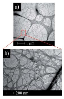
Fig. 1 TEM images of the dispersed MWCNT/CNF sample. Wide range (low magnification) (a) and narrow range (high magnification) images (b).
