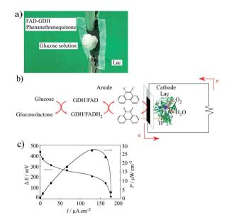
Fig. 7 (a) Photograph of the manufactured actual enzyme-catalyzed biofuel cell with a FAD-GDH bioanode and Lac biocathode. (b) Schematic illustration of the whole reaction of the enzyme-catalyzed biofuel cell. (c) The obtained polarization and power curves of the biofuel cell with 30 mmol dm $^{-3}$  glucose in 0.1 mol dm $^{-3}$  acetate buffer solution (pH 5) at room temperature (15–18 °C).
