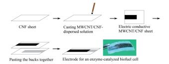
**Scheme 1** Schematic illustration of electrode preparation for the enzyme-catalyzed biofuel cell.
