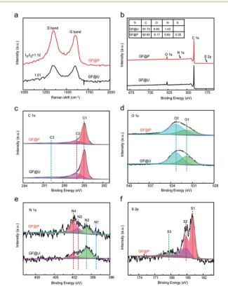
Fig. 3 (a) Raman spectra of GF@U and GF@P of electrode materials. (b) XPS spectra of GF@U and GF@P. (c-f) High-resolution of C1s, O1s, N1s and S2p for GF@U and GF@P.
