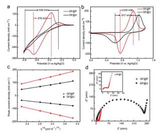
Fig. 4 (a) and (b) Cyclic voltammetries of  $V^{3+}/V^{2+}$  and  $VO^{2+}/VO_2^+$  redox using GF@U and GF@P electrodes at a scan rate of 10 mV s $^{-1}$ . (c) The relationship between GF@U and GF@P peak current density and square root of sweep speed. (d) Impedance diagram of GF@U and GF@P
