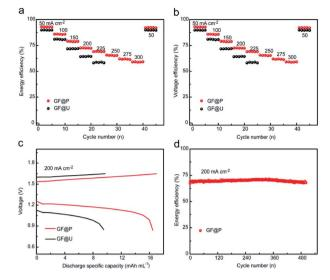
Fig. 5 Charge and discharge performance of VRFBs using GF@U and GF@P electrodes. (a) Energy efficiency. (b) Voltage efficiency. (c) Charge-discharge curves of VRFBs at current density of 200 mA cm<sup>-2</sup>. (d) Long cycle test of GF@P assembled batteries at 200 mA cm<sup>-2</sup>.
