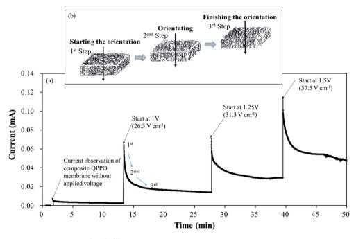
Fig. 7 Effect of the electrical treatment on cQPPO: (a) graph of the current changes according to the elapsed time under a different potential; (b) degree of the alignment with the elapsed time during the fabrication process using an electric field and going in a through-plane direction.
