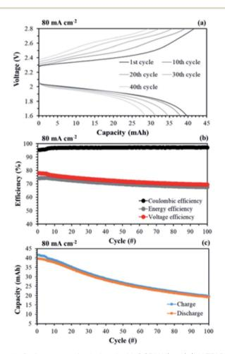
Fig. 17 Performances of a single cell with  $0.05 \, \text{M V}(\text{acac})_3/1 \, \text{M TEABF}_4$  at a high flow rate (120 mL min<sup>-1</sup>): (a) capacity–voltage curves; (b) efficiencies and (d) capacity changes of long-term operation, by applying the aligned cQPPO at 1.5 V.
