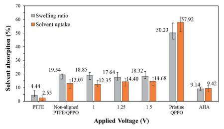
Swelling ratio and solvent uptake for the fabricated membranes in ACN, according to the intensity of the electrical treatment.
