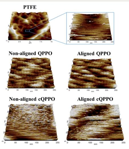
Fig. 13 Morphological AFM image of fabricated membranes: (a) the porous PTFE; (b) empty space of porous substrate; (c) casting QPPO; (d) aligned QPPO at 31 V cm<sup>-1</sup>; (e) non-aligned and (f) Aligned cQPPO at 1.5 V (about 31 V cm<sup>-1</sup>).
