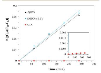
Fig. 19 Comparison of the concentration changes in  $V(acac)_3$  on the deficient side with the elapsed time for the three types of membranes.
