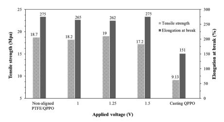
Tensile strength and elongation at break for fabricated membranes in accordance with the applied electrical treatment.
