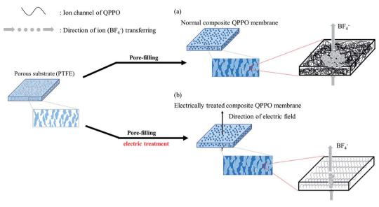
Fig. 1 Process of fabricating the cQPPO membrane: (a) the general fabrication method of the cQPPO membrane and tortuous ion channels of the QPPO polymer, (b) electrically treated QPPO membrane with aligned ion channels of the QPPO polymer in the substrate.
