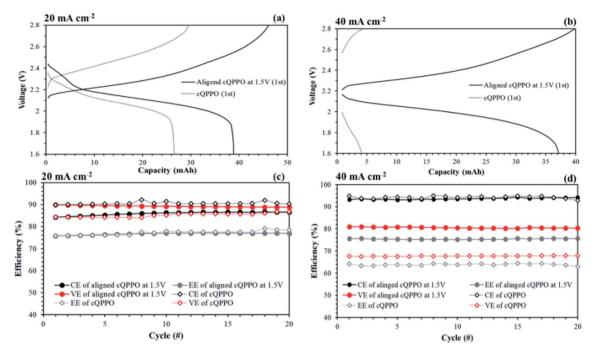
Fig. 15 Comparison of performances in a single cell using  $0.05 \text{ M} \text{ V}(\text{acac})_3/\text{TEABF}_4$  at  $60 \text{ mL min}^{-1}$ : (a) charge/discharge curves at (a) 20 and (b) 40 mA cm<sup>-2</sup>; efficiencies at (c) 20 and (d) 40 mA cm<sup>-2</sup> by applying the non-aligned and aligned cQPPO membrane.
