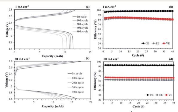
Fig. 16 Comparison of performances in a single cell using 0.05 M V(acac)<sub>3</sub>/TEABF<sub>4</sub> at 60 mL min<sup>-1</sup>: (a) charge/discharge curves and (b) efficiencies by applying AHA membrane; (c) charge/discharge curves and (b) efficiencies by introducing the aligned cQPPO membrane at 1.5 V.
