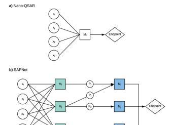
Fig. 1 The schematic representation of the structure-activity prediction networks for modeling of ENMs' toxic activity; x – descriptor that describes either structural attributes (D) or properties (P) of ENMs, M meta-model (meta-models of the 1st layer – indicated in green, and meta-models of the 2<sup>nd</sup> layer – indicated in blue).
