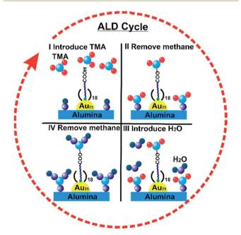
Fig. 11 General scheme of alumina deposition over Au<sub>25</sub>(MUA)<sub>18</sub>/ Al<sub>2</sub>O<sub>3</sub> by atomic layer deposition. Reprinted with permission from ref. 111. Copyright 2018 American Chemical Society.
