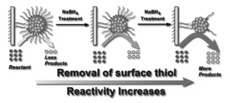
Fig. 7 Illustration of enhanced catalytic activity in a selective oxidation reaction with supported thiolate-stabilized Au<sub>25</sub>(SR)<sub>18</sub> cluster catalysts by mild chemical stripping of their surface ligands with NaBH<sub>4</sub>. Reprinted with permission from ref. 82. Copyright 2014 John Wiley and Sons.
