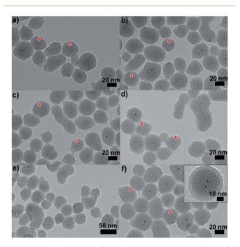
Fig. 9 TEM images of Au<sub>25</sub>@SiO<sub>2</sub> materials calcined at (a) 250 °C, (b) 350 °C, (c) 450 °C, (d) 550 °C, and (e) and (f) 650 °C (inset: enlarged image). Reproduced with permission of the Royal Society of Chemistry. 100
