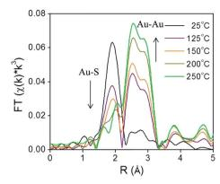
Fig. 4 Au  $L_3$  edge EXAFS spectra in the R space of  $Au_{25}(SR)_{18}$  clusters on carbon (with no phase shift correction). Reprinted with permission from ref. 54. Copyright 2013, American Chemical Society.
