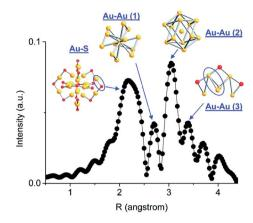
Fig. 2 Simulated FT-EXAFS of  $Au_{25}(SR)_{18}$  clusters. The simulation was done by averaging the EXAFS from all representative Au sites of  $Au_{25}$  (k: 3–14.5 Å $^{-1}$ ,  $k^1$  weighted). The spectrum was phase-corrected using the Au–S peak. Reprinted with permission from ref. 43. Copyright 2011, American Chemical Society.
