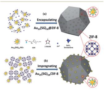
Fig. 10 Illustration of Au<sub>25</sub>(SR)<sub>18</sub> clusters (a) encapsulated in, and (b) impregnated onto, a ZIF-8 metal-organic framework. Reproduced with permission from ref. 110. Copyright 2018 John Wiley and Sons.
