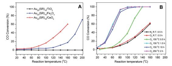
Fig. 3 Activation of Au<sub>25</sub>(SR)<sub>18</sub> clusters over different metal oxides for CO oxidation. (A) CO activity over different metal oxides as a function of temperature for unactivated clusters, and (B) CO activity on ceria supports under different activation conditions. Reprinted with permission from ref. 49. Copyright 2012, American Chemical Society.
