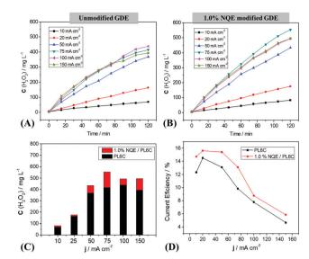
**Fig. 3** (A) Electrogenerated  $H_2O_2$  concentration at different current densities on the unmodified GDE and (B) on the 1.0% NQE modified GDE; (C) comparison of the maximum concentration obtained in 120 minutes of electrosynthesis; and (D) current efficiency of all the densities investigated in 0.1 mol  $L^{-1}$  K<sub>2</sub>SO<sub>4</sub> electrolyte, pH = 2.5 (H<sub>2</sub>SO<sub>4</sub>) under 0.2 bar O<sub>2</sub> pressure.
