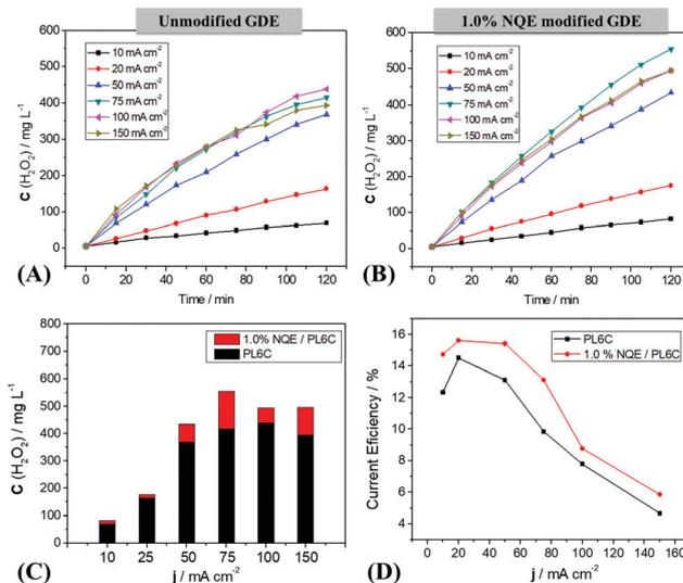
Fig. 3 (A) Electrogenerated  $H_2O_2$  concentration at different current densities on the unmodified GDE and (B) on the 1.0% NQE modified GDE; (C) comparison of the maximum concentration obtained in 120 minutes of electroynthesis; and (D) current efficiency of all the densities investigated in 0.1 mol L<sup>-1</sup>  $K_2SO_4$  electrolyte, pH = 2.5 ( $H_2SO_4$ ) under 0.2 bar  $O_2$  pressure.
