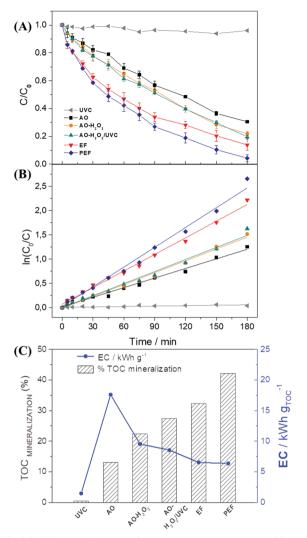
Fig. 5 (A) Effect of different AEOPs on PRM degradation in 180 min of experiment at j=75 mA cm $^{-2}$  using the 1.0% NQE modified GDE with 0.1 mol L $^{-1}$  K<sub>2</sub>SO<sub>4</sub> under pH 2 and 0.2 bar of O<sub>2</sub> flow; (B) analysis of the pseudo-first order kinetics; and (C) comparison between the TOC mineralization and energy consumption in each system.
