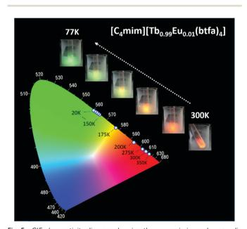
Fig. 5 CIE chromaticity diagram showing the x, y emission color coordinates for  $[C_4\text{mim}][Tb_{0.99}Eu_{0.01}(btfa)_4]$  complexes as a function of temperature with excitation at 360 nm. The inset figures are photographs of the complex at 77 to 298 K taken using a digital camera displaying the green to red emission colors under UV irradiation at 360 nm.
