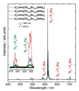
Fig. 4 Emission spectra of the  $[C_4 \text{mim}][Tb_{1-x}Eu_x(btfa)_4]$  (x = 0.01, 0.05, 0.10 and 1.00) complexes recorded at room temperature (300 K), under 360 nm excitation (ligand absorption). The inset shows a magnification of the Tb3+ electronic transitions.
