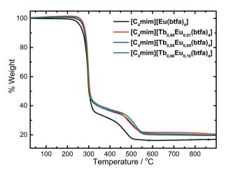
Fig. 1 TGA curves of the  $[C_4 \text{mim}][Tb_{1-x}Eu_x(btfa)_4]$  (x = 0.01, 0.05, 0.10, 1.00) complexes recorded under a synthetic air atmosphere at 10 °C min<sup>-1</sup>.
