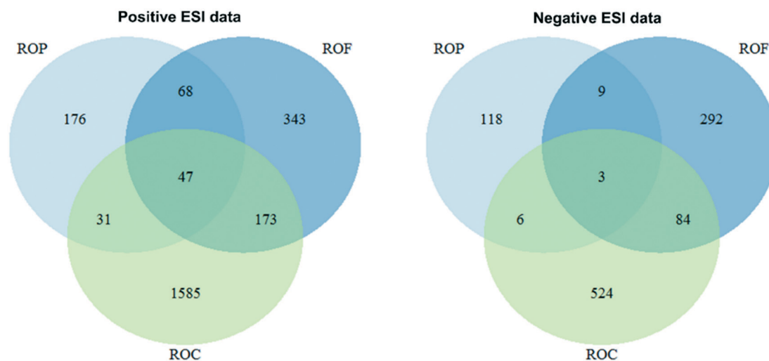
Fig. 2 Venn diagrams of non-target features in samples from the RO drinking water treatment plant detected in positive (left) and negative (right) electrospray ionisation (ESI) datasets. ROF: RO feed water; ROP: RO permeate; ROC: RO concentrate.
