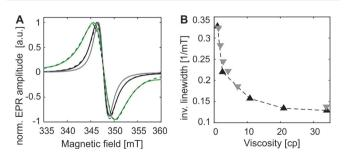
Fig. 1 (A) X-band EPR spectra (T = 293 K) of GDM (grey), GDMA free in solution (black) and bound to eGFP-Y39SCO (green) with Lorentzian fits (dotted lines). (B) Viscosity dependence of the inverse linewidth for GDM (grey) and GDMA (black).
