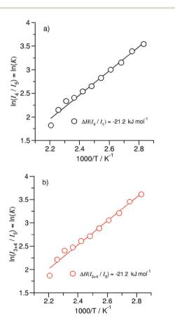
Fig. 7 Plots of the natural logarithm of the ratios (a)  $I_4/I_5$  and (b)  $I_{3+4}/I_5$ versus inverse temperature taken from the deconvoluted spectra in Fig. 6 between 363 K and 453 K. The solid lines represent linear fits ( $R^2 \ge 0.98$ ) with slopes indicating the transfer enthalpies.
