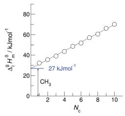
Fig. 2 Measured vaporization enthalpies,  $\Delta_{\rm f}^2 H_{\rm m}^2$ , of alkyl acetates plotted *versus* the total number of carbon atoms ( $N_{\rm C}$ ) in the side chains. The intercept of about 27 kJ mol<sup>-1</sup> at  $N_{\rm C}=0$  gives the contribution of the CH<sub>3</sub> group and allows the correction of the intermolecular HB energy in aliphatic carboxylic acids. The experimental data are taken from Table 2.
