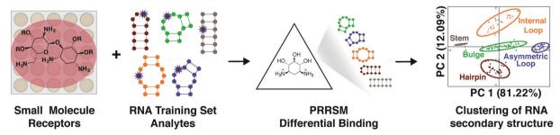
Fig. 5 Pattern recognition of RNA by small molecules (PRRSM). An array of small molecule receptors is titrated with RNA secondary structure analytes. Utilizing the small molecule differential binding and an unbiased statistical method allows for clustering based on the RNA structural motifs. Reprinted with permission from ref. 19. Copyright 2019 American Chemical Society
