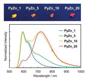
Fig. 3 Normalized emission spectra (lower,  $\lambda_{\rm ex}$  = 370 nm) and image (upper,  $\lambda_{ex} = 365 \text{ nm}$ ) of **PyZn\_R**.
