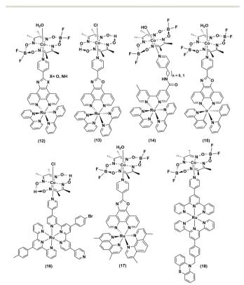
Fig. 3 Noble metal-based photosensitizer-cobaloxime dyads for photocatalytic hydrogen evolution.
