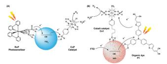
Fig. 9 (A) Schematic representation of photocatalytic  $H_2$  production  $TiO_2$  NPs containing a covalently attached cobalt catalyst (CoP) and a ruthenium photosensitiser (RuP). (B) Representative figure of the photocathode containing organic dye P1 and cobaloxime catalyst Co1 on the NiO surface. The figures are redrawn from ref. 78 and 79 respectively.
