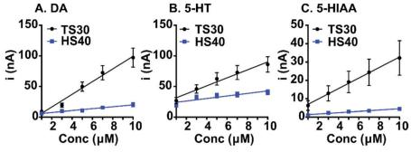
Fig. 3 Sensitivity comparison for TS30 and HS40 fibers. All calibration curves were conducted from 1 μM to 10 μM. (A) Dopamine (waveform: -0.4 V to 1.3 V, 400 V s<sup>-1</sup>, n = 6-10), (B) 5-HT, and (C) 5-HIAA (waveform for TS30: 0.2 V to 1.0 V, down to -0.1 V and back to 0.2 V, 1000 V s<sup>-1</sup>; HS40: -0.4 V to 1.3 V, 400 V s<sup>-1</sup>, n = 8-10).
