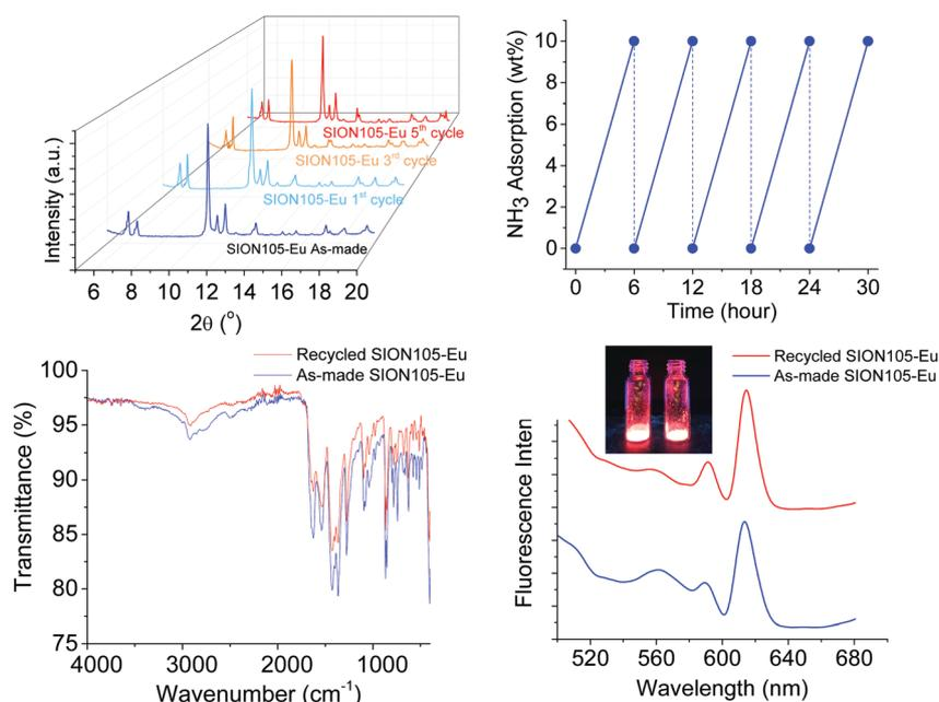
Fig. 3 (top left) PXRD patterns of **SION105-Eu** after recycling cycles; (top right) the  $\text{NH}_3$  vapour adsorption capacity of the MOF remains the same after 5 cycles; (bottom) FTIR spectra and luminescence emission ( $\lambda_{\text{ex}} = 360\text{ nm}$ ) of the as-made and recycled **SION105-Eu**. The inset shows the red emission under UV radiation of the as-made (left) and recycled (right) materials.
