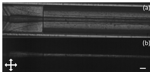
Fig. 5 Jetting of a core of RO-TN 651 within a sheath of 12.5% PI in n -hexane and a coagulation bath of 7% LiBr and 10% PVP in ethanol, as viewed between (a) uncrossed polarisers and (b) crossed polarisers. The birefringent jet in (b) comes from the jetting of the RO-TN. Scale bar 200 \mu\text{m} . Flow rates are 1.25 \text{mL h}^{-1} bath, 0.45 \text{mL h}^{-1} polymer, and 0.60 \text{mL h}^{-1} liquid crystal.
