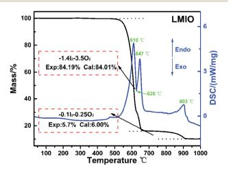
Fig. 2 TG and DSC analyses of LMIO.
