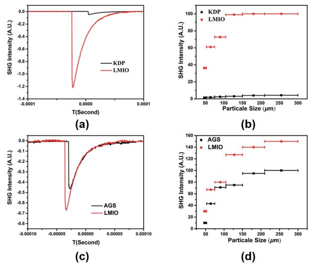
Fig. 4 Oscilloscope traces of the SHG signal (150–210 mm) of LMIO at (a) 1064 nm and (c) 2.05  $\mu$ m. Plots of measured SHG intensity vs. particle size of LMIO under laser radiation at (b) 1064 nm and (d) 2.05  $\mu$ m. KDP and AGS samples serve as the references for 1064 and 2.05  $\mu$ m laser radiation, respectively.
