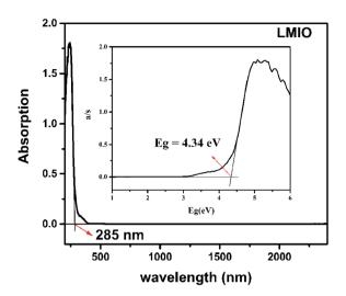
Fig. 3 UV-Vis-IR analysis of LMIO.
