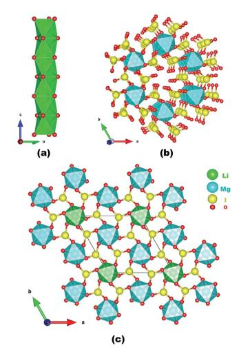
Fig. 1 A 1D chain of face-sharing  $LiO_6$  octahedra along the c-axis (a); the 3D  $[Mg(IO_3)_6]^{4-}$  anionic framework along the c-axis (b); and the view of the structure of LMIO along the c-axis (c).
