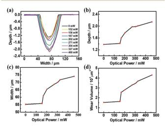
Fig. 5 (a) Cross-sectional profiles, (b) depths, (c) widths, and (d) removal volumes of the concave microlens fabricated on an n-GaAs wafer under different illumination powers. The imprint time is 15 minutes, and the aqueous solution contains 40 mM KMnO<sub>4</sub> and 1.84 M H<sub>2</sub>SO<sub>4</sub>
