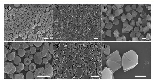
Fig. 2 SEM images of nanostructures of R-SPAn in different  $f_w$ : (a and b) 50%, (c and d) 85% and (e and f) 90%, respectively. ([R-SPAn] = 1.5 mM, scale bar 1  $\mu$ m). Upon increasing the fraction of water, the morphologies transformed from 0D nanospheres with a rough surface or with a hole to 2D and finally to 3D layered nanoflakes.
