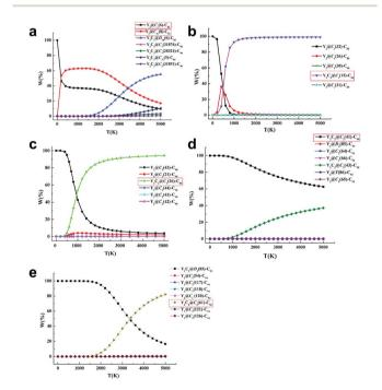
Fig. 4 Computed molar fraction as a function of temperature for the low-lying isomers of (a)  $Y_2C_{82}$ , (b)  $Y_2C_{88}$ , (c)  $Y_2C_{90}$ , (d)  $Y_2C_{92}$ , and (e)  $Y_2C_{94}$ . The isomers marked with red boxes are experimentally obtained.
