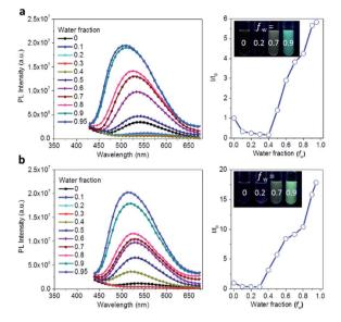
Fig. 5 Aggregation-induced emission effect of the TSCT-HABs. PL spectra and the relative emission intensity of Ac3TRZ3 (a) and TAc3TRZ3 (b) in THF/water mixed solvents at a concentration of 1  $\times$  $10^{-5}$  mol L<sup>-1</sup>; inset: PL images with different water fractions ( $f_w$ ) under UV light (365 nm).
