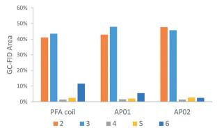
Fig. 12 Distribution between the desired product 2, quenched starting material 3 and the side products 4, 5 and 6 according to GC-FID obtained from reactions at 0 °C in three different reactors (AP01 = cascade, AP02 = split and recombine reactor).
