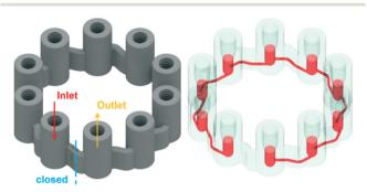
Fig. 2 CAD drawing of the micro CSTR cascade (AP01). (Left) View from outside with indication of the blocked parts and resulting in-/ outlet vessels. (Right) Exposed channels and vessels of the cascade.
