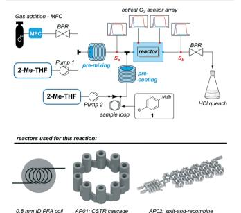
Fig. 11 General scheme of the reaction set-up to carry out the aerobic oxidation of 1 in three different reactors including the positioning of the optical oxygen sensors.
