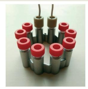
Fig. 6 3D printed CSTR cascade (APO1) closed with standard HPLC fittings. The 3D printed 10-32 UNF thread had to be refined after the printing.
