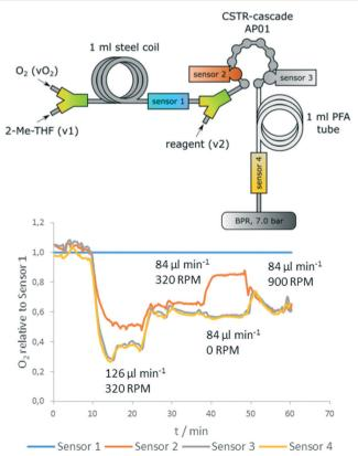
Fig. 10 Flow setup with sensor arrangement in the reactor (top); relative oxygen content in the reactor at varying reagent flow rate v2 (1 M 4-methoxyphenylmagnesium bromide). vO2: 1500 μl min<sup>-1</sup>, v1: 1000  $\mu$ l min<sup>-1</sup> (bottom).
