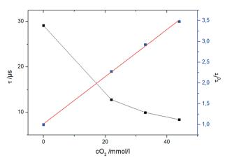
Fig. 9 Evaluation of the oxygen calibration with the fibre sensor in THF at 0 °C and oxygen concentrations up to 42 mmol L<sup>-1</sup>.
