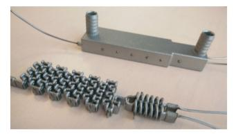
Fig. 7 3D printed split and recombine reactor (APO2) for the oxidation of Grignard reagents with and without cooling shell. After postprocessing, 1/16" capillaries were welded to the in- and outlets for connection with standard HPLC equipment.
