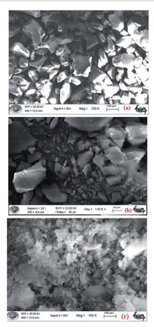
Fig. 3 SEM images of the (a) activated silica gel (Si), (b) Si-CPTS adsorbent and (c) Si-CPTS-AHAP adsorbent.
