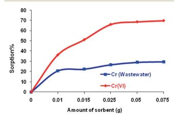
Fig. 8 The effect of the amount of sorbent on the sorption of Cr(vı) from aqueous solution and wastewater.
