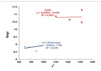
Fig. 11 The D-R isotherms for the adsorption of Cr(vi) from agueous solution and wastewater by the Si-CPTS-AHAP adsorbent.
