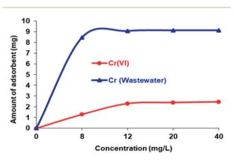
Fig. 5 The adsorption effect depends on the concentrations of Cr(v<sub>i</sub>) in aqueous solution and wastewater.
