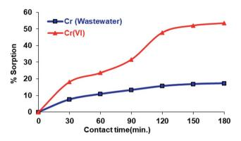
Fig. 7 The effect of the contact time on the adsorption of Cr(v) from aqueous solution and wastewater.
