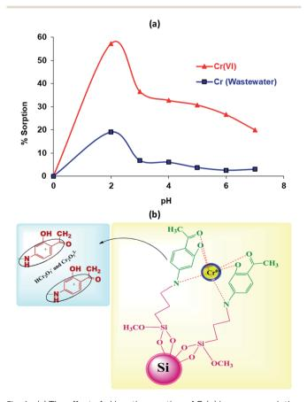
Fig. 4 (a) The effect of pH on the sorption of  $Cr(v_l)$  in aqueous solution and wastewater. (b) Si-CPTS-AHAP  $Cr(v_l)$  metal ion combination and a schematic of the electrostatic attraction of acetophenone to  $HCl_2O_7^{-}$  and  $Cr_2O_7^{2-}$  anions.
