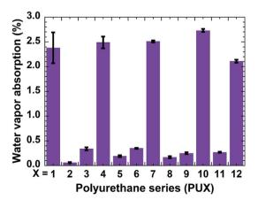
Fig. 5 Water vapor absorption of PU1-12 coatings.
