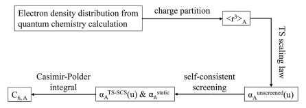
Fig. 1 Flow diagram for TS-SCS method.
