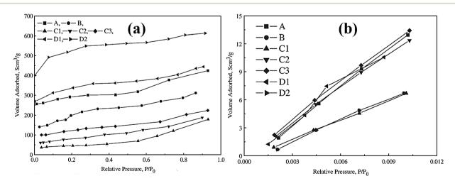
Fig. 1  $N_2$  and  $CO_2$  adsorption isotherms of the activated carbon produced from different starting materials. <sup>26</sup> This figure has been adapted from ref. 26 with permission from Elsevier.
