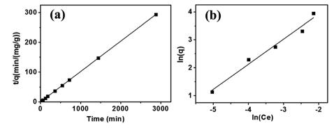
Fig. 3 (a) Pseudo-second order model for Hg sorption (pH 6, adsorbent 80 mg L<sup>-1</sup>, Hg<sup>2+</sup> 1.0 mg L<sup>-1</sup>, 25  $\pm$  2 °C). (b) Freundlich isotherm model for Hg sorption (Hg<sup>2+</sup> 0.5–5.0 mg L<sup>-1</sup>, pH 6, adsorbent 80 mg L<sup>-1</sup>, time 24 h, 25  $\pm$  2 °C). This figure has been adapted from ref. 37 with permission from Elsevier.
