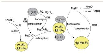
Fig. 4 Schematic diagram of the mechanisms of Hg(n) removal by *in situ* Mn-Fe.<sup>55</sup> This figure has been adapted from ref. 55 with permission from Elsevier.
