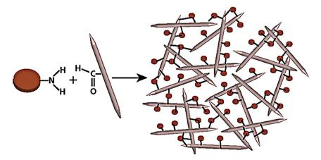
Fig. 7 Schematic of the preparation of the chemically crosslinked CNC/GQD hydrogel.<sup>95</sup> This figure has been adapted from ref. 95 with permission from ACS Nano.
