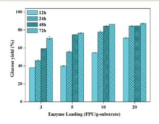
Fig. 4 Glucose yield as the function of enzymatic hydrolysis time with different enzyme loading (CCR pretreated with 16 wt% of KOH at 70  $^{\circ}$ C for 90 min; enzymatic hydrolysis solid loading of 15% at 50  $^{\circ}$ C).
