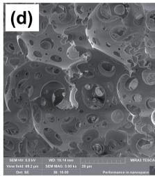
Fig. 1 SEM images of (a) OSP before calcination, (b) OSP after calcination at 900 °C, (c) foam, and an (d) enlarged view of (c).
