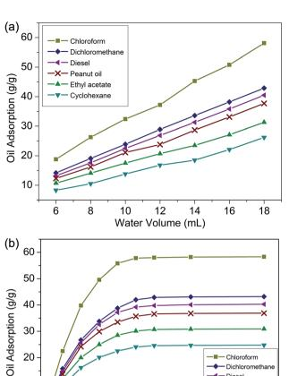
10 20 30 40 50 60 Time (s) Fig. 6 (a) Oil adsorption of foams with different amounts of water: (b) adsorption kinetics of foams
