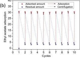
Fig. 7 (a) Centrifugation for the extraction of ethyl acetate (dyed with Sudan II for clear observation); (b) oil adsorption capacities in different cycles.
