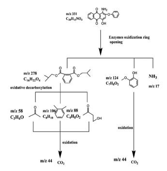
Fig. 11 Degradation pathway analysis of Disperse Red 3B.
