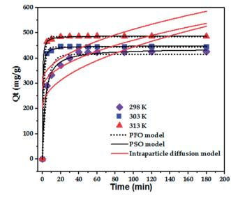
Fig. 5 Nonlinear fit models: PFO, PSO, and IPD.
