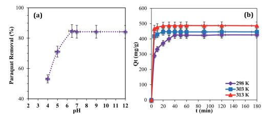
Fig. 4 (a) Effect of initial solution pH (T = 298 K;  $C_i = 100$  mg L<sup>-1</sup>; m = 20 mg). (b) Effect of contact time (temperature: 298, 303, and 313 K;  $C_i = 100$  mg L<sup>-1</sup>; m = 20 mg; pH = 6.5).
