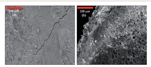
Fig. 2 SEM photographs of (a) jujube seed and (b) JS/HSO-700.
