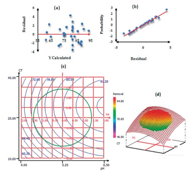
Fig. 9 Normality test: (a) plot of raw residuals vs.  $Y_{calculated}$ ; (b) probability as a function of residual and (c) contour plots (2D and 3D presentations).
