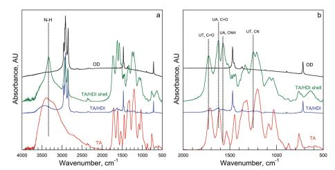
Fig. 4 FTIR spectra from OD, TA, and TA/HDI (both the OD-filled PH and the PUU shell): (a) spectra from 500 to 4000 cm<sup>-1</sup>; (b) spectra from 500 to 2000 cm<sup>-1</sup> showing the main urethane and urea bands.
