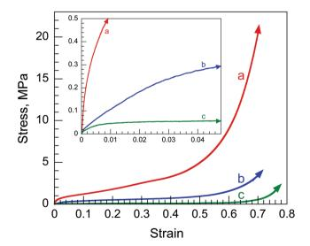
Fig. 7 Compressive stress-strain curves from: (a) TA/HDI; (b) TA/TDI; (c) TA/N75. Inset: enlargement of the results at low strains.
