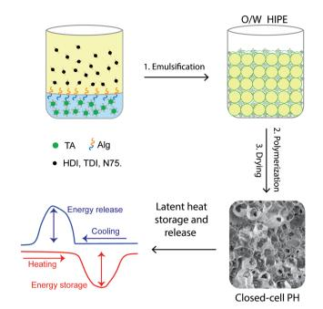
**Fig. 1** A scheme illustrating the synthesis of PCM-encapsulating PHs for thermal energy storage and release applications through ISGP within a HIPE.
