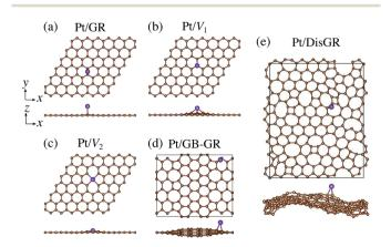
Fig. 1 Optimized structures of Pt single-atom adsorption on (a) pristine graphene (GR), (b) graphene with a carbon mono-vacancy  $(V_1)$ , (c) graphene with a carbon di-vacancy ( $V_2$ ), (d) grain-boundary graphene (GB-GR), and (e) disorder graphene (DisGR)
