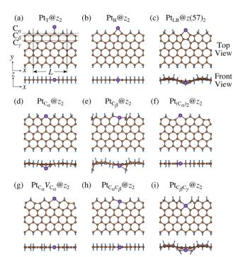
Fig. 6 Optimized structures of Pt single-atom adsorption at the edges of di-hydrogenated zGNRs. Purple, brown, and light blue spheres represent Pt, C, and H atoms, respectively. The first, second, and third outermost C atoms are denoted as  $C_{\alpha}$ ,  $C_{\beta}$ , and  $C_{\gamma}$ , respectively. L indicates the periodicity of the ribbons along the edge direction.
