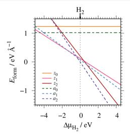
Fig. 2 Formation energy of GNR as a function of H $_2$  chemical potential.  $\Delta\mu_{\rm H_2}=\mu_{\rm H_2}-E_{\rm H_2}$ , where  $E_{\rm H_2}$  is the total energy of a gas-phase H $_2$  molecule at 0 K.
