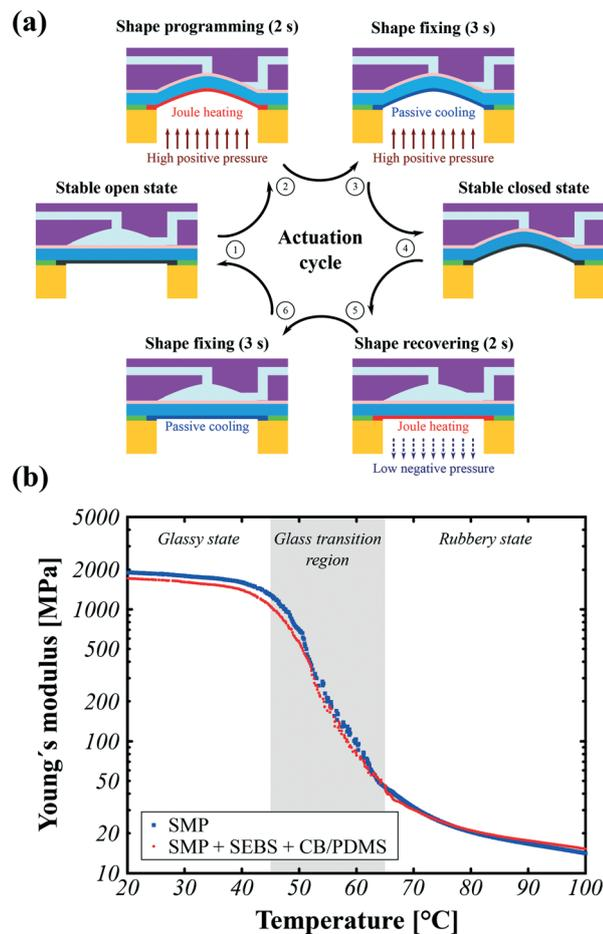
Fig. 2 Working principle of our SMP valves. (a) Schematic illustration of the complete valve actuation cycle (open  $\rightarrow$  closed  $\rightarrow$  open). By combining pneumatic pressure and Joule heating, each valve can be cyclically open and closed. (b) Measured Young's modulus versus temperature for the SMP material used as a single thin layer and in the tri-layer.
