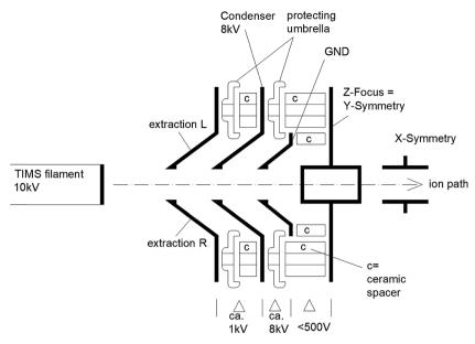
Fig. 5 Simplified schematic representation of a TIMS ion source (not to scale).
