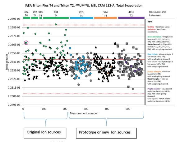
Fig. 8 QC chart displaying total evaporation <sup>235</sup>U/<sup>238</sup>U data collected on NBL 112-A certified reference material with various ion sources on the IAEA TIMS Triton Plus 'T4' and Triton 'T2'. Pink circled measurement discussed in Fig. 3.
