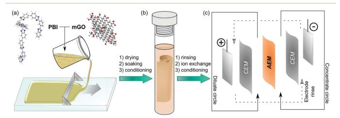
Fig. 1 Schematic fabrication to application overview of the nanocomposite AEMs based on modified GO and quaternised polybenzimidazole (PBI): membrane casting of the PBI-mGO blend (a), methylation of PBI (b) and electrodialysis with AEM (c).
