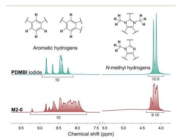
Fig. 5  $\,^{1}$ H NMR spectra of PDMBI iodide and M2-0 membrane showing aromatic and N-methyl hydrogens. The area ratios of the signals show 100% and 50–60% quarternisation of the benzimidazole groups for PDMBI and M2-0, respectively.
