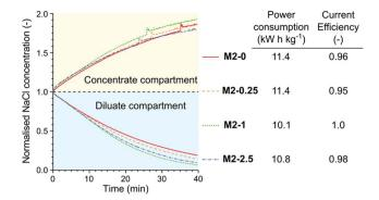
Fig. 11 The concentration curves, power consumption of NaCl removal and current efficiency in the electrodialysis of 0.1 M NaCl solution with different M2 membranes.
