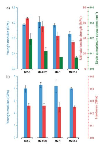
Fig. 8 Mechanical properties of the M2 membranes obtained by (a) tensile testing and (b) nanoindentation.
