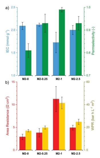
Fig. 9 (a) Electrochemical properties (ion exchange capacity and perm selectivity) and (b) resistive properties (Area Resistance and Water Permeation Resistance) of the M2 membranes.
