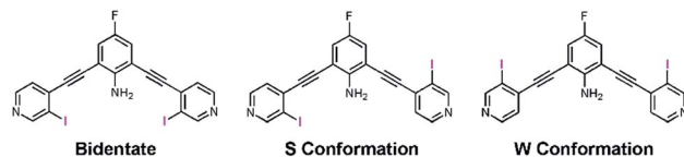
Fig. 2 ChemDraw representations of the three planar conformations obtained by rotating about the alkyne bonds: the bidentate conformation (left), where both XB donors are convergent; the S conformation (middle), where the XB donors are on opposite sides of the molecule; and the W conformation (right), where both XBs are directed away from the amine.
