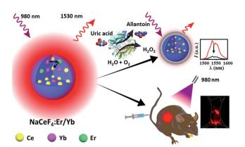
Scheme 1 Schematic illustration showing *in vitro* bioassays and *in vivo* bioimaging based on NaCeF<sub>4</sub>:Er/Yb nanoprobes.
