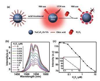
Fig. 3 (a) Process and principle of homogeneous assay of  $H_2O_2$  by employing NaCeF4:Er/Yb as the probe. (b) NIR-II emission spectra of ligand-free NaCeF<sub>4</sub>:Er/Yb NCs after the addition of different concentrations of  $H_2O_2$  upon excitation at 980 nm. (c) Calibration curve for the  $H_2O_2$  assay. The inset shows the linear range (0.078–10  $\mu$ M) of the calibration curve.
