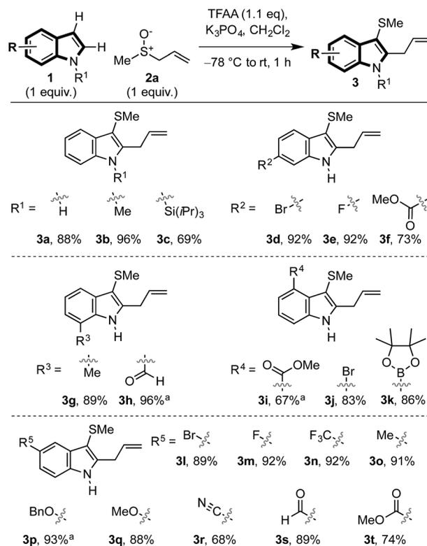
Scheme 2 Exploring the scope of indoles in the dual vicinal functionalisation cascade. <sup>a</sup> 1.5 equivalents of sulfoxide and 1.6 equivalents of TFAA were used.
