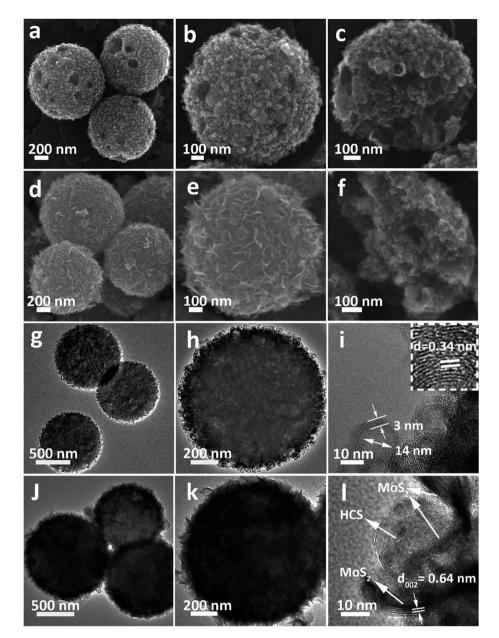
Fig. 1 (a-c) FESEM, (g and h) TEM and (i) HRTEM images of the HCSs. (d-f) FESEM, (j and k) TEM, and (l) HRTEM images of the  $MoS_2@HCS$  composite.
