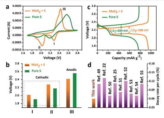
Fig. 5 (a) CV curves, (b) discharge-charge curves and (c) the comparison of the peak voltages of the pure S and  $MoS_2 + S$  electrodes. (d) A comparison of the decay rate per cycle with that of other Li-S cathode materials reported in the literature recently.
