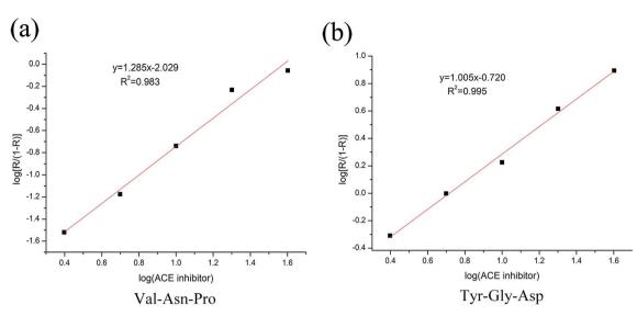
Fig. 8 Inhibition curve of Val-Asn-Pro standard (a). Inhibition curve of Tyr-Gly-Asp standard (b)
