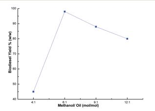
Fig. 9 Effect of methanol/oil ratio on biodiesel yield.
