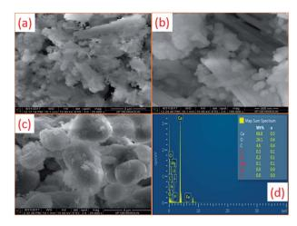
Fig. 4 SEM images of (a) and (b) uncalcined and (c) calcined snail shells as well as (d) the EDS spectra of calcined shells at  $900 \, ^{\circ}$ C for 4 h.
