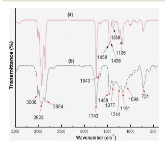
Fig. 12 FT-IR spectra of (a) soybean oil biodiesel and (b) soybean oil.
