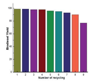
Fig. 14 Reusability of nanoparticles for the transesterification reaction. Operating conditions: catalyst loading of 3 wt% (w/w); methanol to oil ratio of 6 : 1 (m/m); reaction time of 7 h.
