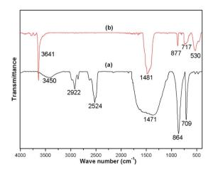
Fig. 3 FTIR of (a) snail shells (b) snail shells calcined at  $900 \, ^{\circ}\text{C}$  for 4 h.
