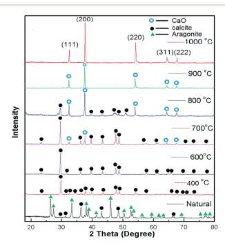
Fig. 1  $\,$  XRD patterns of natural snail shells and calcined snail shells of different temperatures ranging between 400 to 1000  $^{\circ}\text{C}$  for 4 h.
