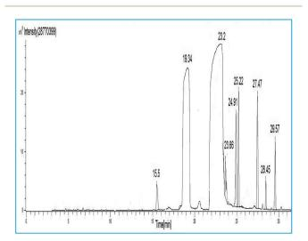
Fig. 13 GC-MS spectrum of soybean oil biodiesel.
