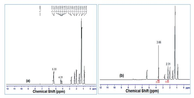
Fig. 11 <sup>1</sup>H-NMR spectroscopy of (a) fresh soybean oil and (b) soybean oil biodiesel.
