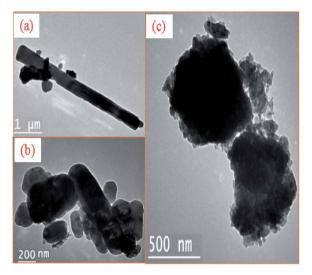
Fig. 5 TEM images of (a) uncalcined and (b) and (c) calcined snail shells
