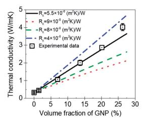
Fig. 8 The thermal conductivity of GNP-PTFE nanocomposites predicted by a modified MGEMA.
