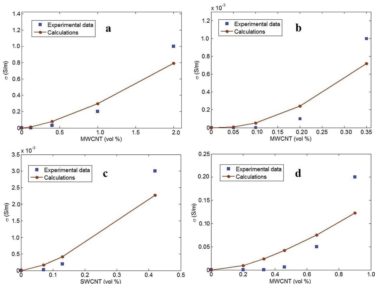
Fig. 2 Experimental results and calculations by the developed model for (a) epoxy/MWCNT,<sup>42</sup> (b) PVC/MWCNT,<sup>43</sup> (c) epoxy/SWCNT<sup>44</sup> and (d) PC/ABS/MWCNT<sup>45</sup> samples.
