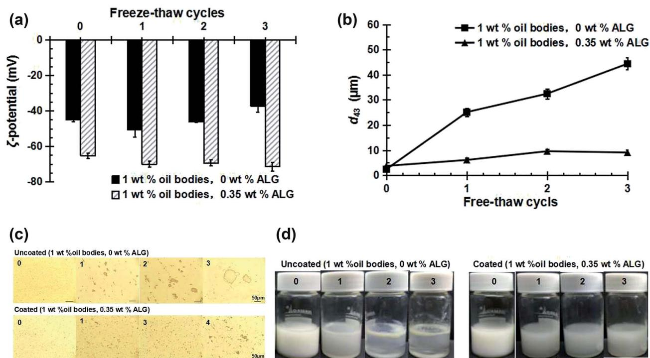
Fig. 7 Effect of freezing–thawing cycling on  $\zeta$ -potential (a); mean particle diameter ( $d_{43}$ ) (b); the microscopic structure (c) and the creaming stability (d) of uncoated (1 wt% oil bodies, 0 wt% ALG) and coated (1 wt% oil bodies, 0.35 wt% ALG) OB emulsions at pH 7. The oil bodies were dispersed in 50 mM sodium phosphate buffer solution. The creaming observation was made after storage at  $22 \pm 2$  °C for 7 days. “0, 1, 2, 3” represents the number of the freezing–thawing cycles.
