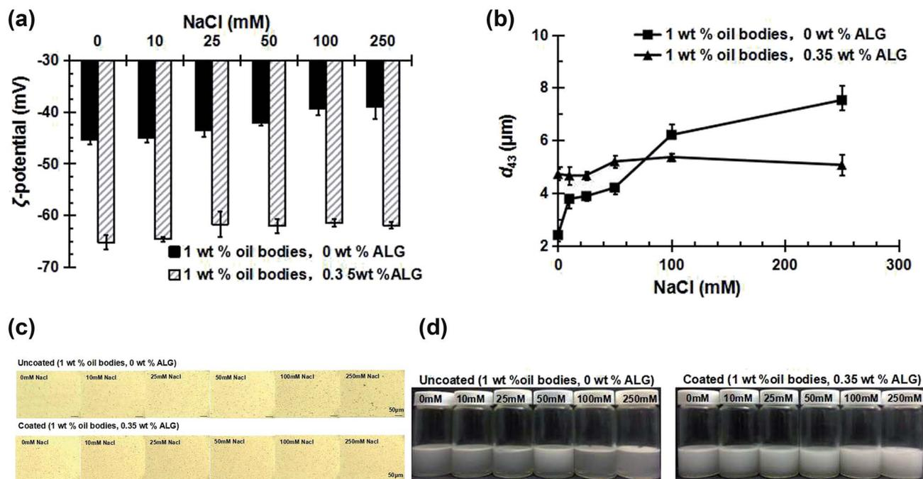
Fig. 6 Salt effect on  $\zeta$ -potential (a); mean particle diameter ( $d_{4,3}$ ) (b); the microscopic structure (c) and the creaming stability (d) of uncoated (1 wt% oil bodies, 0 wt% ALG) and coated (1 wt% oil bodies, 0.35 wt% ALG) OB emulsions at pH 7. The oil bodies were dispersed in 50 mM sodium phosphate buffer solution. The creaming observation was made after storage at  $22 \pm 2$  °C for 7 days.
