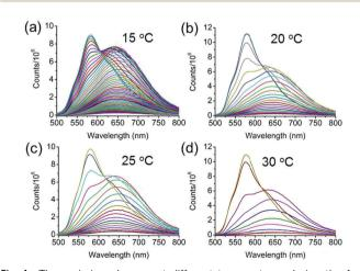
Fig. 4 The emission changes at different temperatures during the formation of the nanorods. (a) 15  $^{\circ}$ C, (b) 20  $^{\circ}$ C, (c) 25  $^{\circ}$ C, and (d) 30  $^{\circ}$ C.  $C_{\text{CTAB}} = 1.0 \text{ mg mL}^{-1}$ . The spectra were recorded every 3 min.
