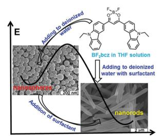
Fig. 1 The image representation of the preparation of the BF<sub>2</sub>bcz nanospheres and nanorods from the BF<sub>2</sub>bcz monomer in THF solution. the morphological transition from nanospheres to nanorods, and the schematic energy diagram depicting the energy barrier between the nanospheres and nanorods
