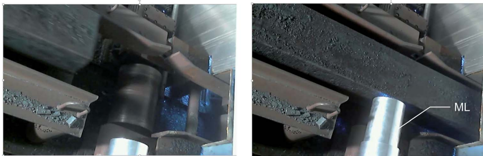
Fig. 7 Inline measurement of steel blooms, left: the bloom is transported on a roller table and arriving from the left, right: the measuring lance (ML) is approached to the side face of the bloom, laser irradiation is activated to locally ablate the scale layer and to analyse the bulk composition. Diameter of ML: 170 mm. 32
