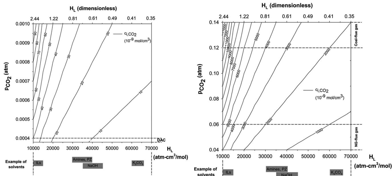
Fig. 25 Interfacial concentration of CO<sub>2</sub>,  $c_i$ , based upon Henry's law for DAC (left) and the flue gas of natural gas and coal (right).
