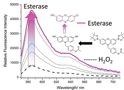
**Fig. 6** Fluorescence spectra of **Pinkment-OAc** ( $0.5 \mu\text{M}$ ) following incubation ( $15 \text{min}$ ) with PLE ( $0.1$ – $0.6 \text{U}$ ) and subsequent addition of  $\text{H}_2\text{O}_2$  ( $1 \text{mM}$ ). The data was collected in PBS buffer ( $100\% \text{w/w H}_2\text{O}$ ) at  $\text{pH} = 7.4$ ,  $25^\circ\text{C}$ .  $\lambda_{\text{ex}} = 545$ – $20 \text{nm}$ . Dashed line represents  $\text{H}_2\text{O}_2$  ( $1 \text{mM}$ ) addition only.
