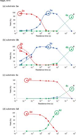
Fig. 1 Tandem isomerizations of various aryl benzyl ethers by changing the residence time in R1 in a flow microreactor system for products 2, 3 and 4d, followed by further stirring in a flask at 50 °C for 1 h to obtain products 4a-c (#). Methyl triflate was used as an electrophile (symbol ▲ with a dashed line), instead of methyl iodide (symbol • with a solid line).
